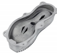
Metal 3D Printed Pop-corn mold
